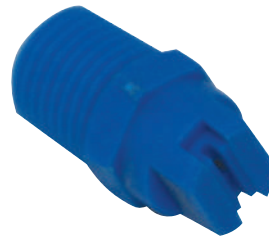
PLASTIC NOZZLE TIP, BLUE, 1/4" NPT 1.0 GPM, 65° Part # 10-250-19-PP For use on CTA
